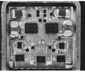
ENLARGEMENT OF A THIN film hybrid microcircuit.
